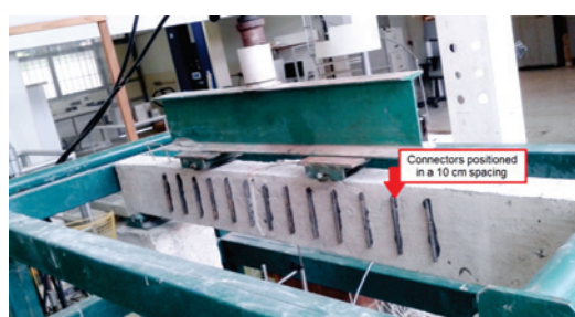
b) Connectors positioned in a 10 cm spacing
