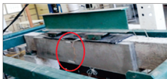
d) Extensometers attached on the sides of the reinforcement (region tensioned and compressed)
