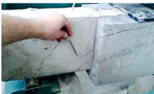
b) Beam support crack due to shearing
