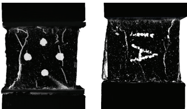
Figure 14 Formation of conical cracks for l/h = 1.0
