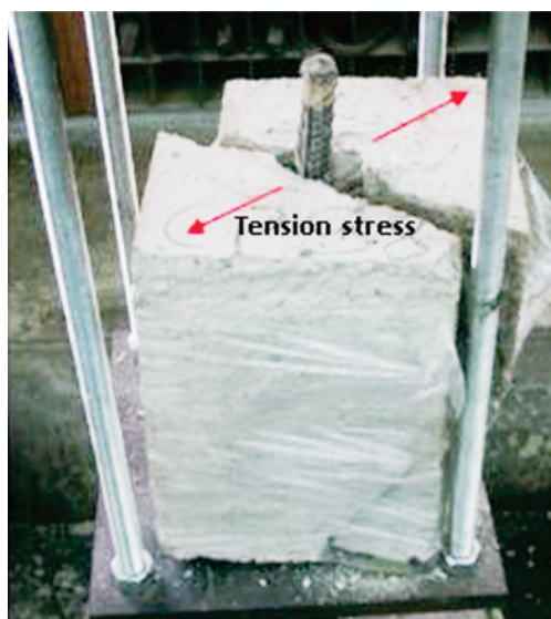
Figure 10 Brittle failure in CR models
