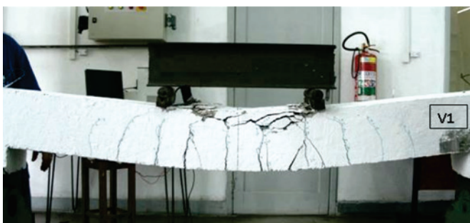
Figure 8 Cracking mode and type of failure of the beams V1 e V2
