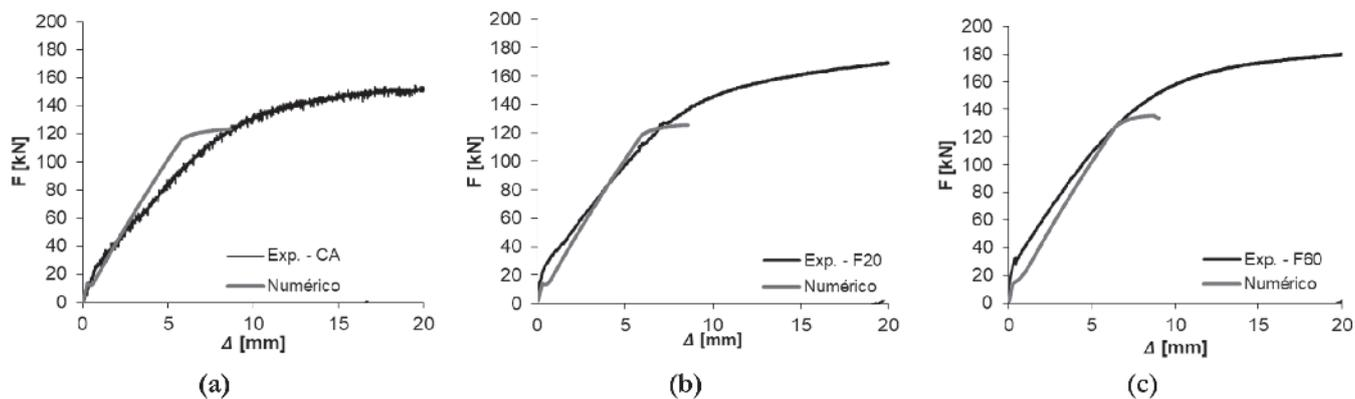
**Figure 15** Comparison of the results: a) RC – no fibers; b) F20 – 20 kg/m<sup>3</sup> of steel fibers, c) F60 – 60 kg/m<sup>3</sup> of steel fibers
