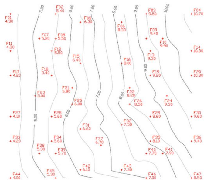
Figure 13 Isosettlement curve of the SHELL SSI model
