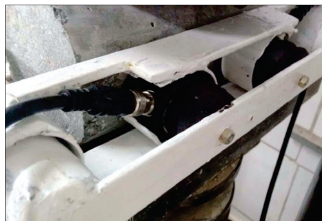
Figure 3 Detail of attaching transducers to tensile diametrical compression test (split test)
