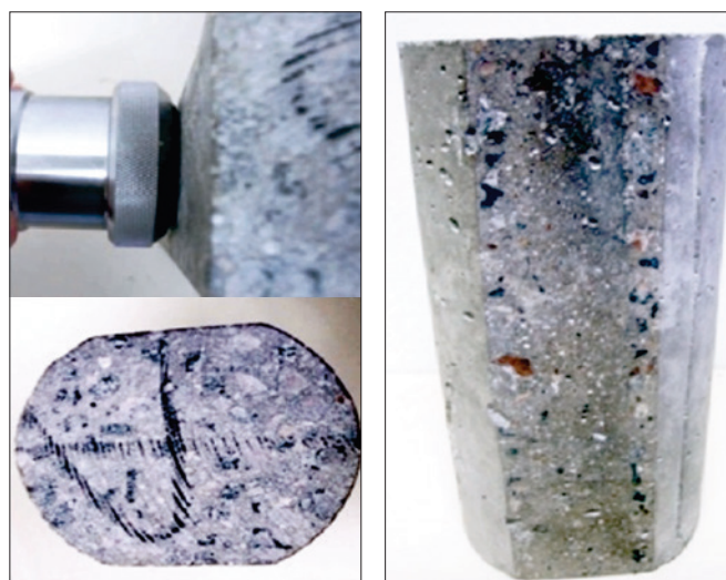
Figure 1 Grinding of specimens to attach transducers
