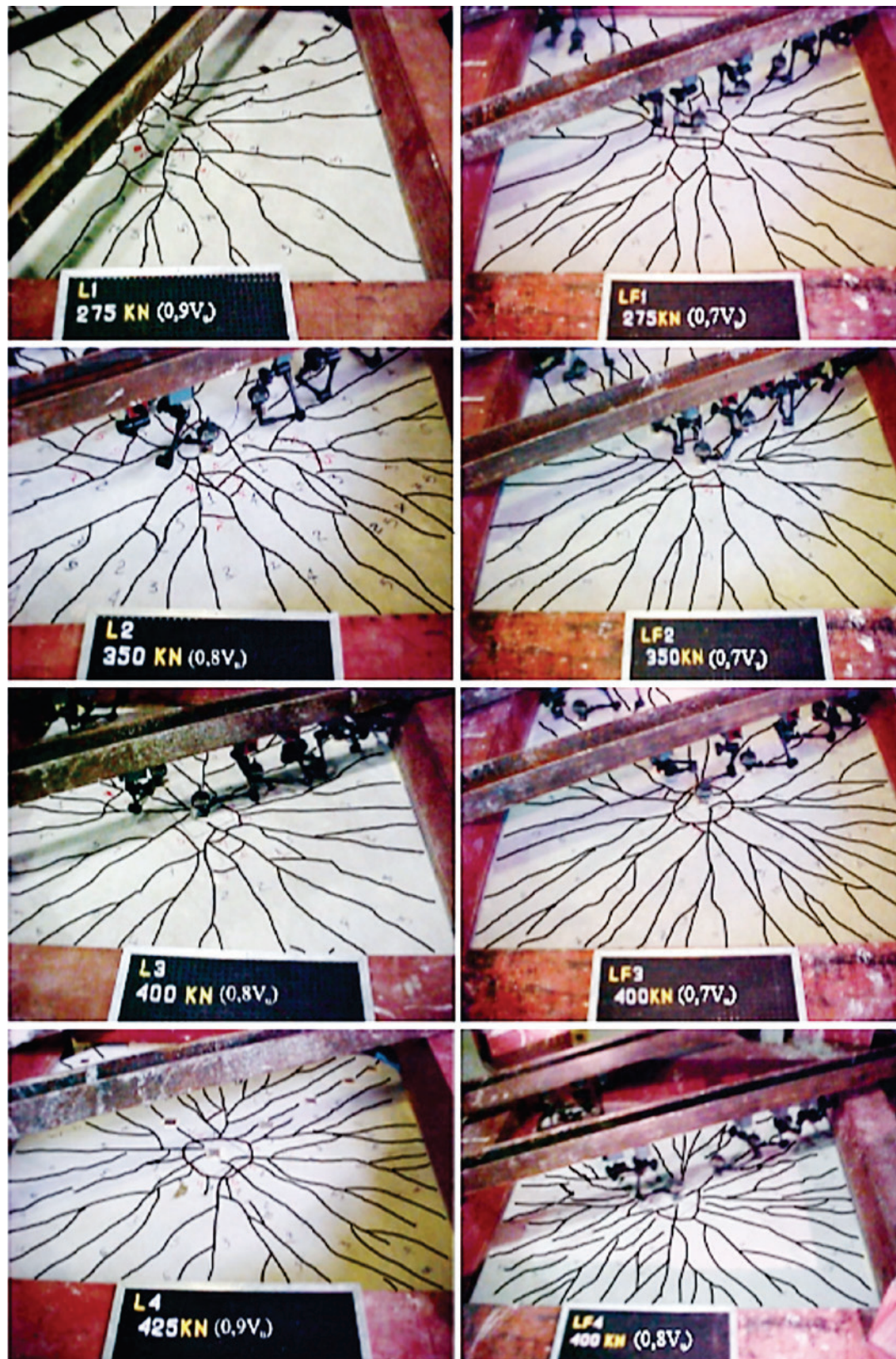
Figure 16 Slab cracking patterns at higher loading stages (70% to 90% of ultimate loads)
