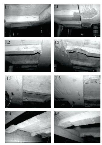
Figure 14 Slabs' failure mode
