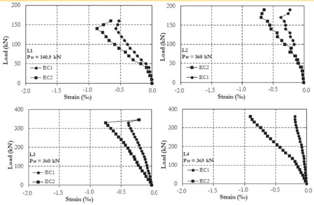
Figure 11 Slabs' concrete strains
