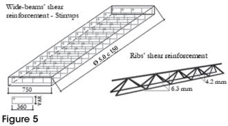
Slabs' trussed shear reinforcement
