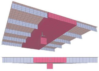
Figure 15 Slab's model with 250 mm depth wide-beam
