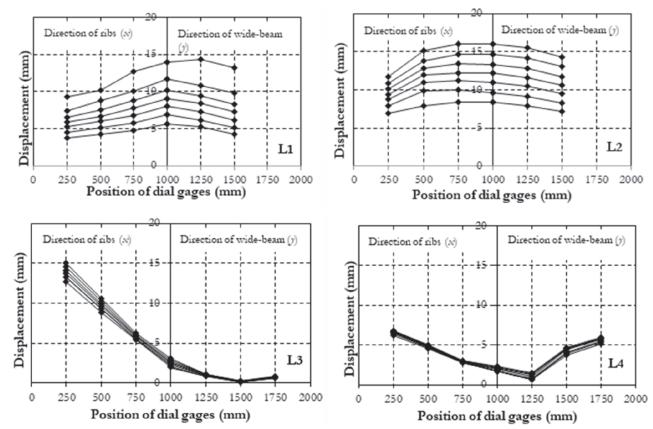
Figure 10 Displacements along the length of the slabs
