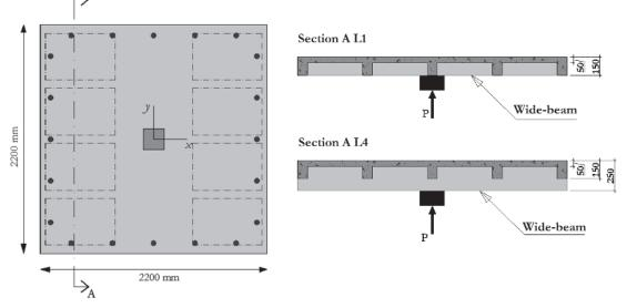
Figure 3 Slabs' dimensions of the series under study
