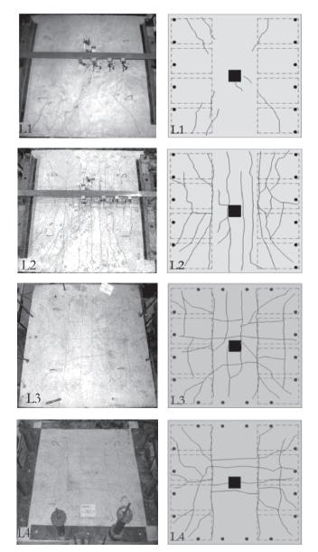
Figure 13 Slabs' cracking pattern
