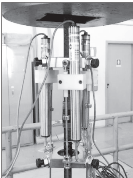
Figure 12 Transducers in groups of three installed on the fixed triangular steel bases used in test method 3
