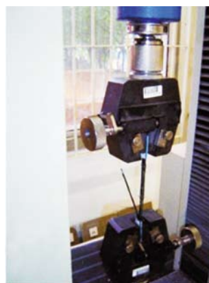
Break of CFRP in tensile tests
