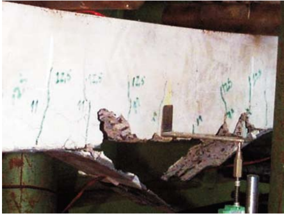
Break of CFRP – VR 01
