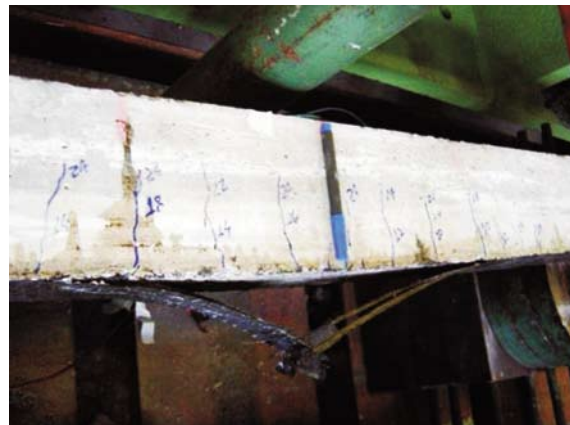
Break of CFRP – VR 10
