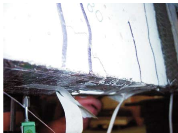
Break of CFRP – VTF5
