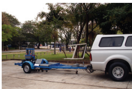
Figure 2 – FWD tests over transversal joints
