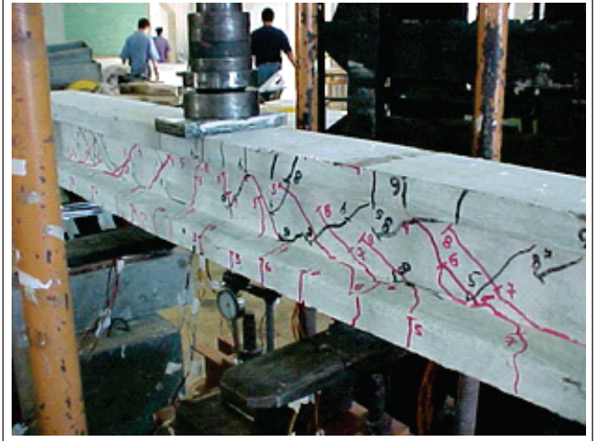
Figure 3 – Detailed view of cracking in beam I80-BC30-I
