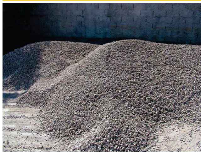
Figure 3 – Melt shop Slag , deposited in the courtyard of Reciclos company in Timóteo-MG
