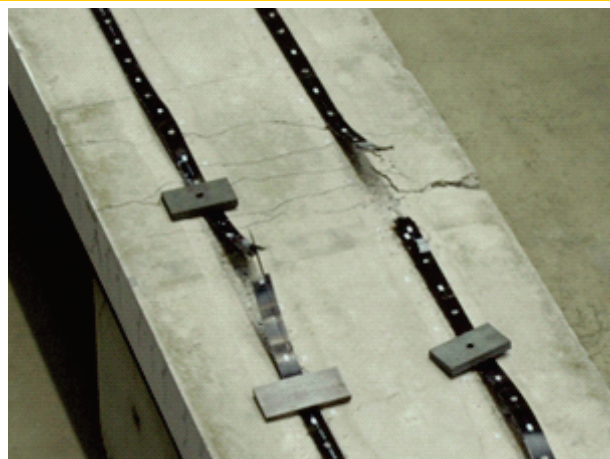
Figure 4 – Failure of post-strengthening strips: (a) Next to a flexural crack; (b) Distant from flexural cracks
